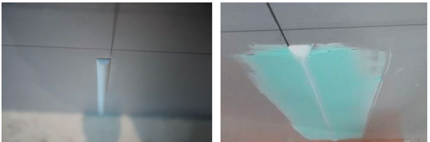
Figure 3: Picture of the untreated welding seam (left) and the faired welding seam (right) used for towing tank experiments.
