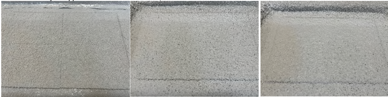
Figure 2 A) Mist coat of Hempatherm IC 175 (0.5 mm WFT) B) Light coat of Hempatherm IC 175 (1-2 mm WFT) C) Subsequent coat(s) of Hempatherm IC 175 (2-3 mm WFT)
