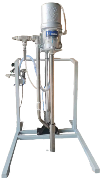
Photo C4. Pneumatically operated height adjustable mount on a Graco President.
