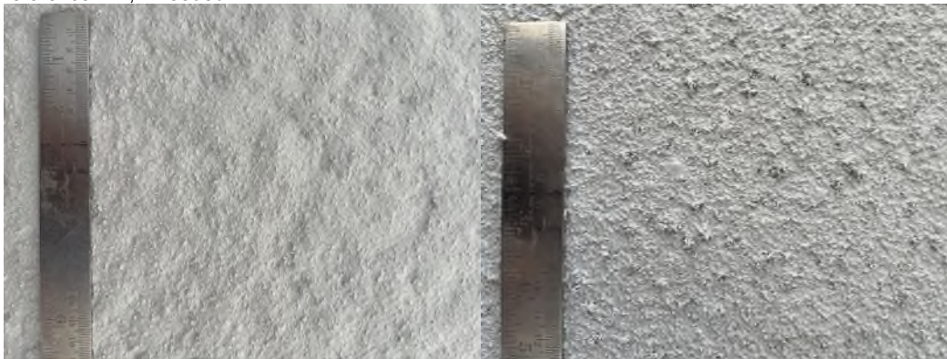
Figure 3 Examples of good uniform finish and of poor rough finish from Hempterm IC 170 spray application.
