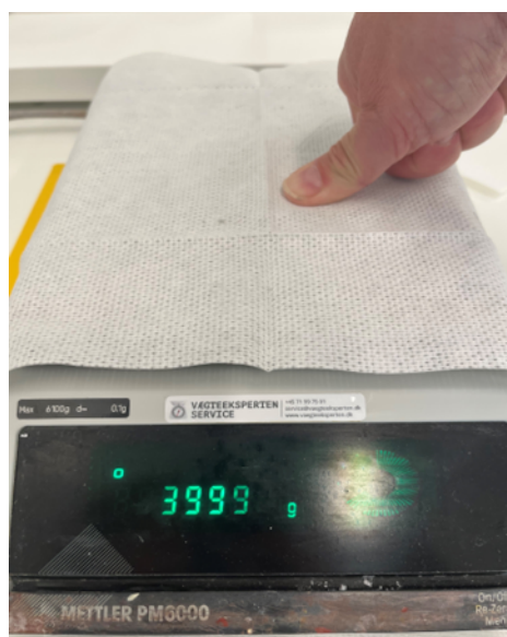
Picture 2: Thumb calibration to check the amount of pressure that corresponds to 4Kg
